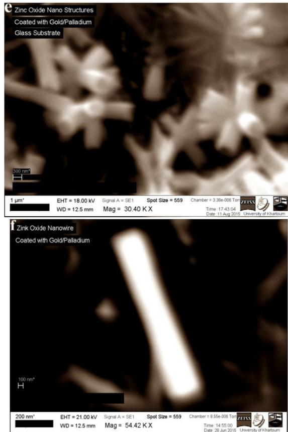
**Figure 2 (a) ZnO tetrapods and flower like structures at  $\mu\text{m}$ , (b) ZnO multipods with size 300 nm, (c) ZnO closed multipods with spherical shape and flower like structure, (d) ZnO spherical closed multipods at 300 nm, (e) ZnO open tetrapods at 300 nm, ZnO nanorods at 100 nm scale.**
