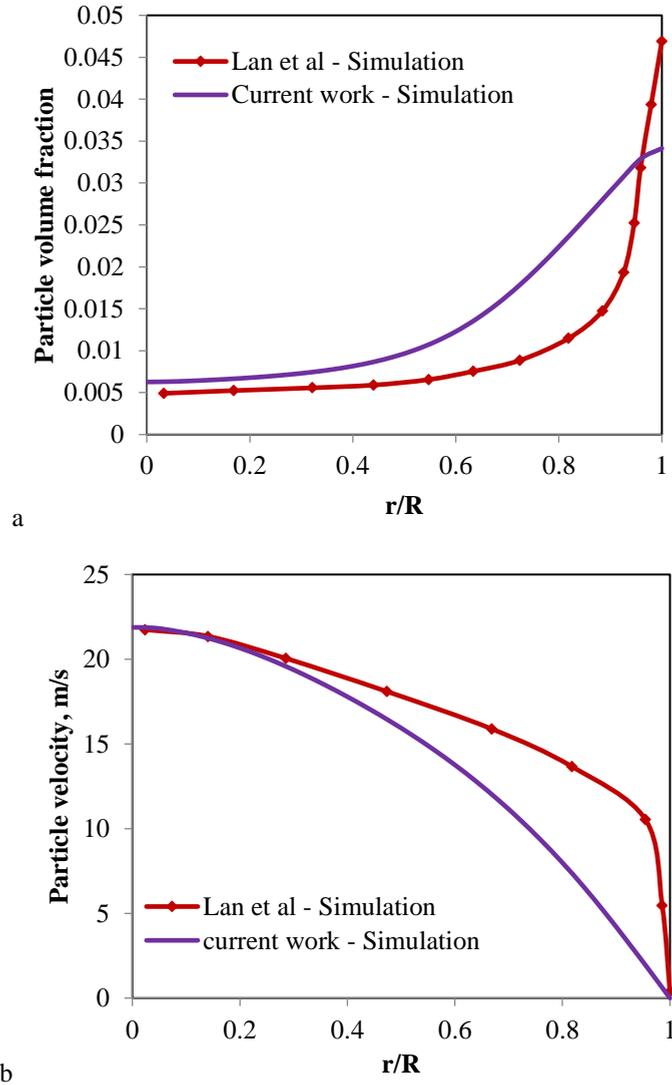
Figure 4: Comparison of particle volume fraction (a) and particle velocity (b) at the riser outlet between the predicted model and simulation results of Lan *et al.* [11]
