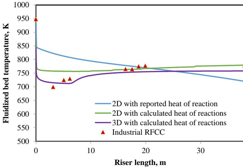
Figure 5: Comparison of solid phase static temperature profile resulted from simulation cases of 2D and 3D models when using reported and calculated heat of reactions
