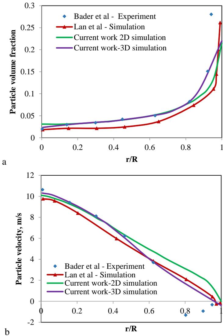
Figure 2: Comparison of particle volume fraction (a) and particle velocity (b) at the 4 m riser level between the predicted models and the experimental data of Bader *et al.* [14]
