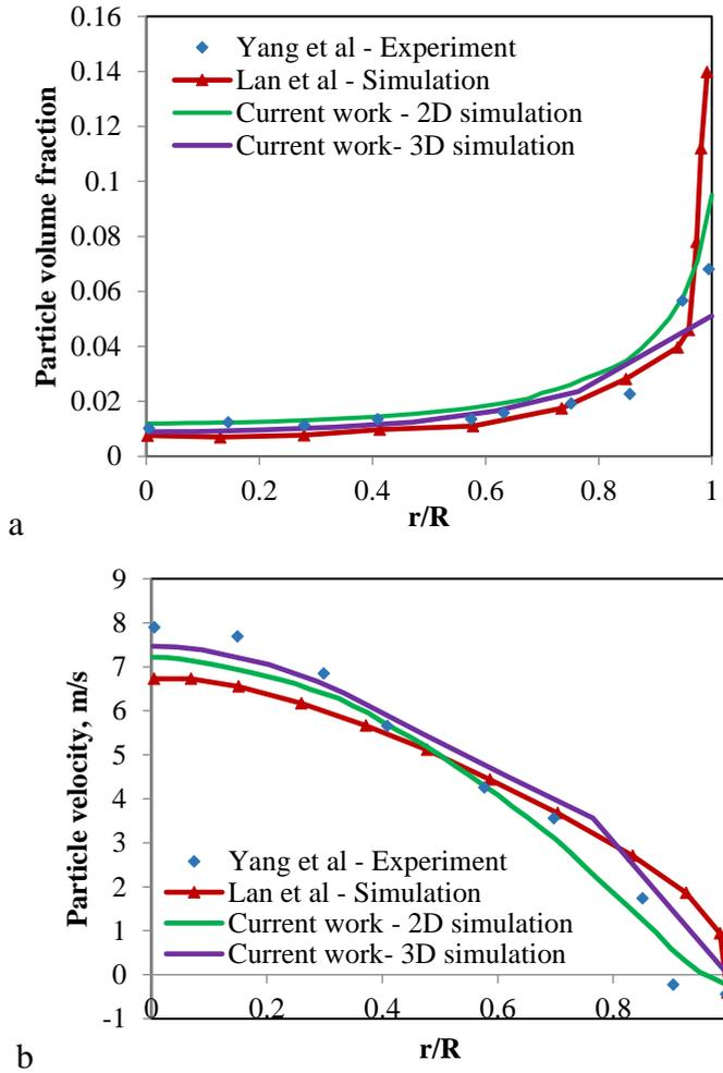
Figure 1: Comparison of particle volume fraction (a) and particle velocity (b) at the 5.6 m riser level between the predicted models and the experimental data of Yang [21]
