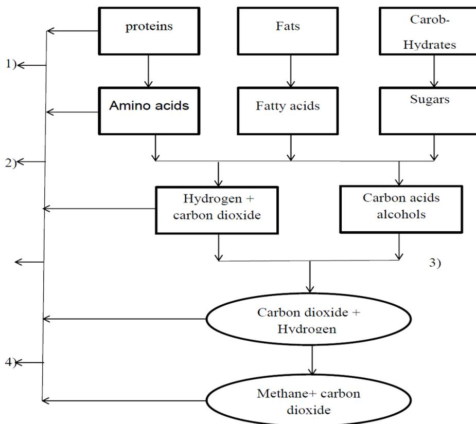
**Figure 1 the main process of anaerobic digester**
