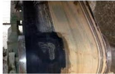
Figure-2: Belt Damage
